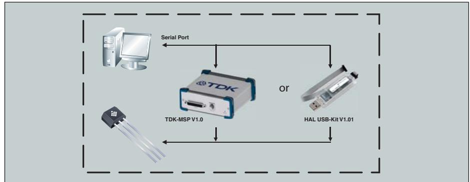
Fig. 1: Development tool setup for HAL 1880 and HAL 1890
