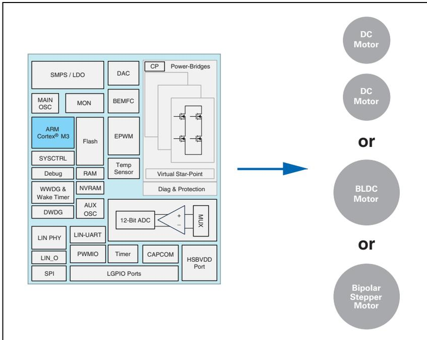
Fig. 1: Motor control applications with HVC 4420F
